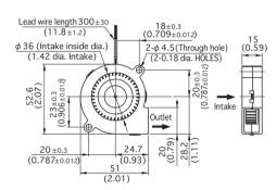
Lead wire spec. UL1061 AWG26 or UL3265 AWG26 Color (+) Red (-) Black
